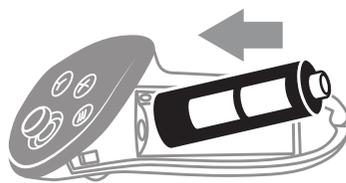
NOTE: Ensure the charging contacts are facing out as shown in the drawing.
