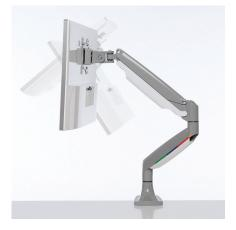
One-Touch Monitor Arm with Built-In Gas Spring gives you total control over your monitor's position through effortless adjustment of its height, depth and angle 170 - 505mm height adjustment, ±90° swivel and monitor rotation and ±90° tilt adjustment.
