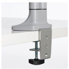
Easy, Non-permanent Installation mountable by C-clamp (desktop thickness 10 - 85mm) or grommet (desktop thickness 10mm - 80mm, grommet hole diameter 10.5 - 50mm). Installation is non-permanent and non-marking and includes tool kit for easy removal.
