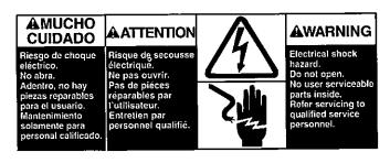
This means an electrical shock hazard exists if covers, enclosures or guards are removed and internal parts become accessible. ALWAYS refer servicing to qualified GBC service personnel.
