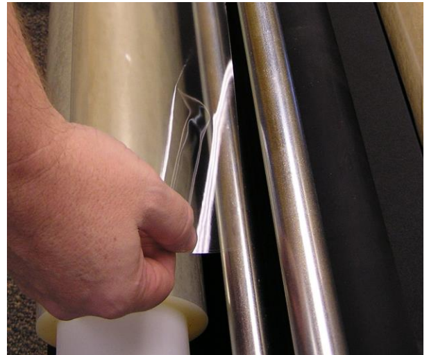
Start the bottom leader between the rubber rollers using the foot pedal
